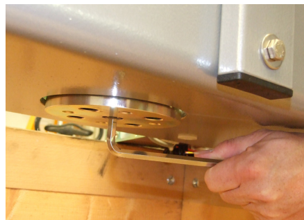
Fig. 15: Turn the screw on the drive shaft
