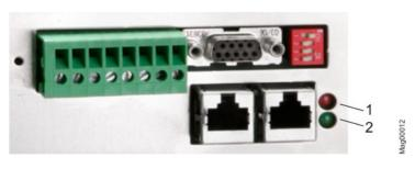
Fig. 25: LEDs on MMC-120
