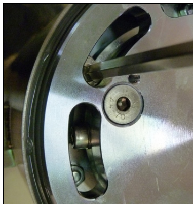
Fig. 17: Adjusting the left end stop
