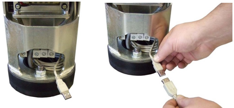
Fig. 27: Connect the laptop to the control unit MBC-111.
