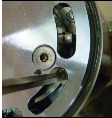
Fig. 16: Adjusting the right end stop
