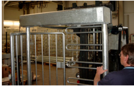
Fig. 14: Mounting the support beam
