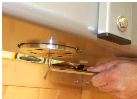
Fig. 20: Turn the screw on the drive shaft
