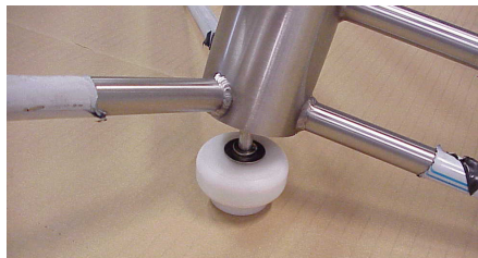
Fig. 27: Place the center column on the floor bearing
