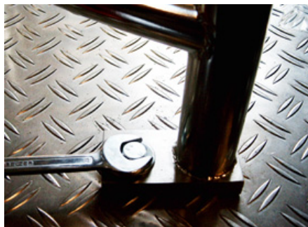
Fig. 16: Tighten the fastening screws
