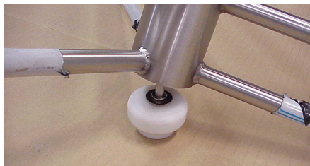
Fig. 22: Place the center column on the floor bearing
